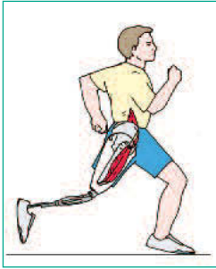
Figure 3. Sound Limb Stride – reaching out with sound limb for an equal stride length
